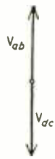
Fig. 6. This alternative to Fig. 4(b) identifies the voltages on the circuit diagram unambiguously without any arrows at all.
